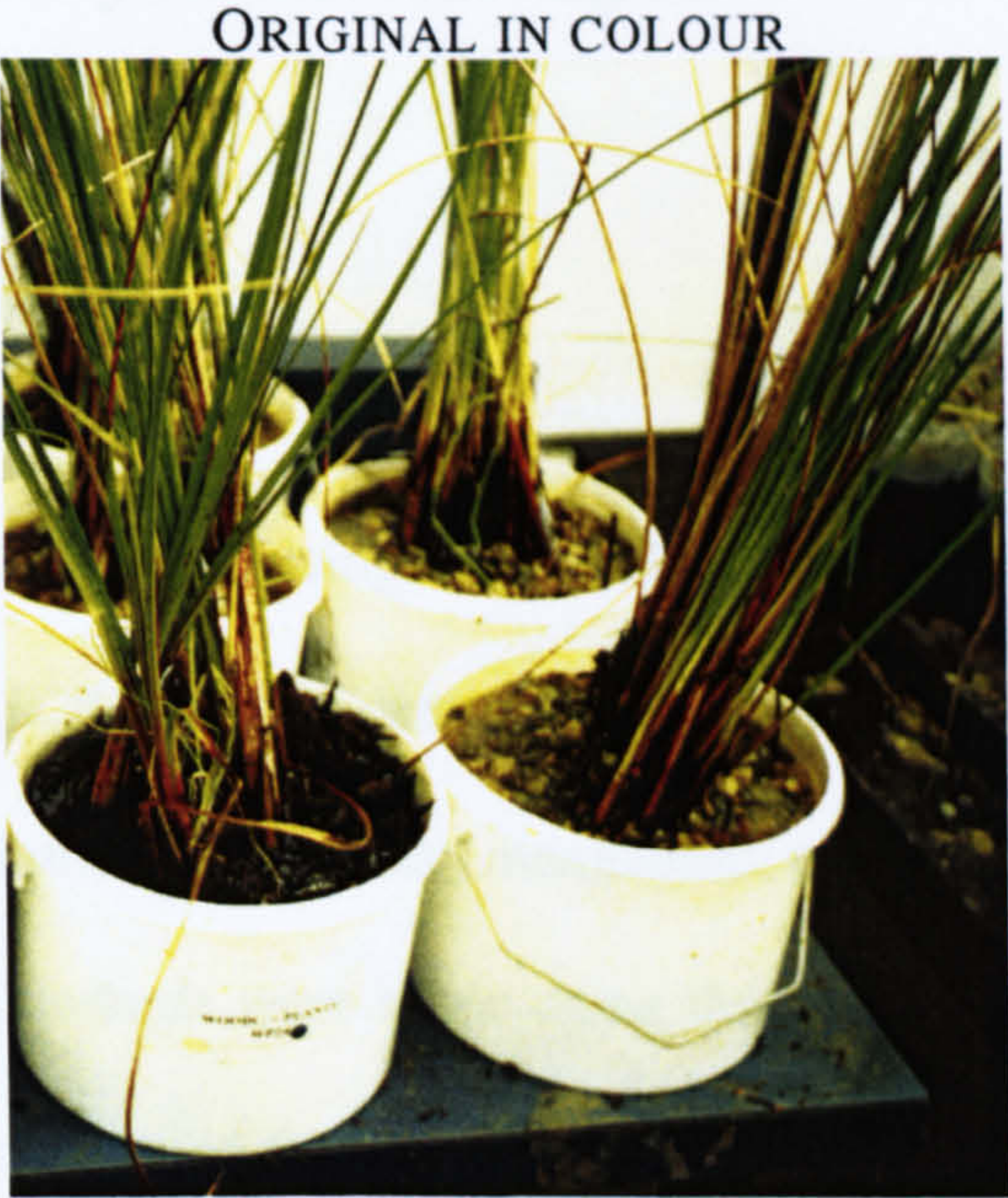
Figure 2.8: An example of planted microcosm set up, treating mine drainage water.
